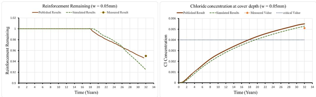
Fig.1 – Chloride concentration and reinforcement remaining ratio for crack width of 0.05 mm.
