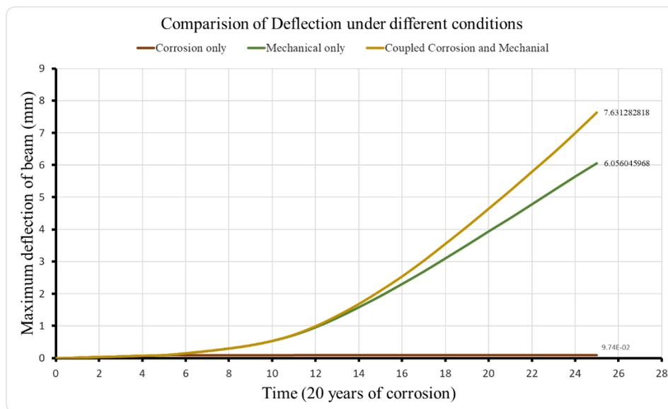
Fig.2 – Deflection under different case of loading.
