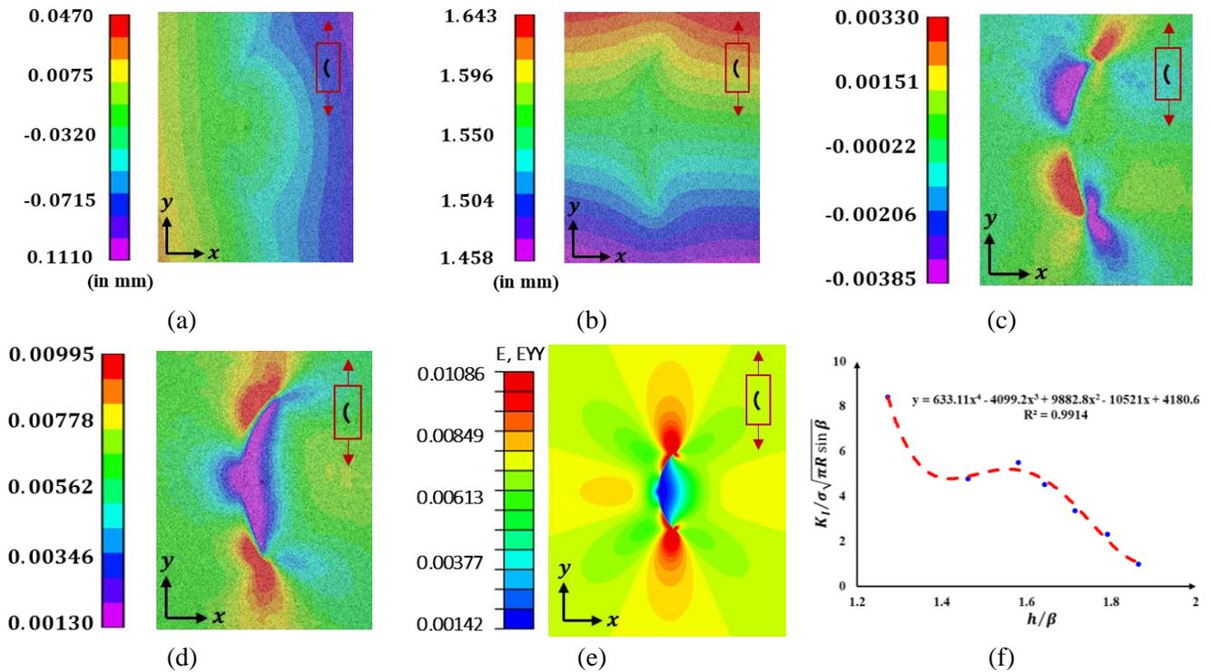
Fig. 2. Displacement and strain contours obtained using DIC and FEA simulation. (a)  $u_x$  (b)  $u_y$  (c)  $\epsilon_{xy}$  (d)  $\epsilon_{yy}$  (e) FEA contours (f) variation of normalized SIF with respect to  $(h/\beta)$  ratio
