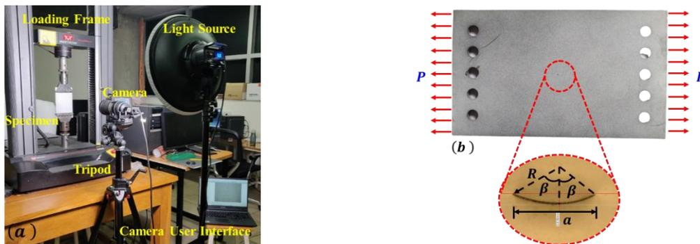
Fig. 1. Experimental setup and actual specimen (a) Experimental Setup (b) Specimen sprayed with speckle pattern
