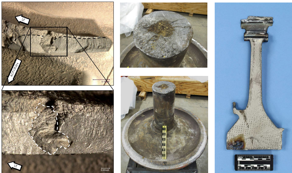
Figure 1. Turbocharger turbine wheel fractured blade (left images), rail car axle fracture with central void (middle images), and HPT stage 2 disk fracture surface (right image).
