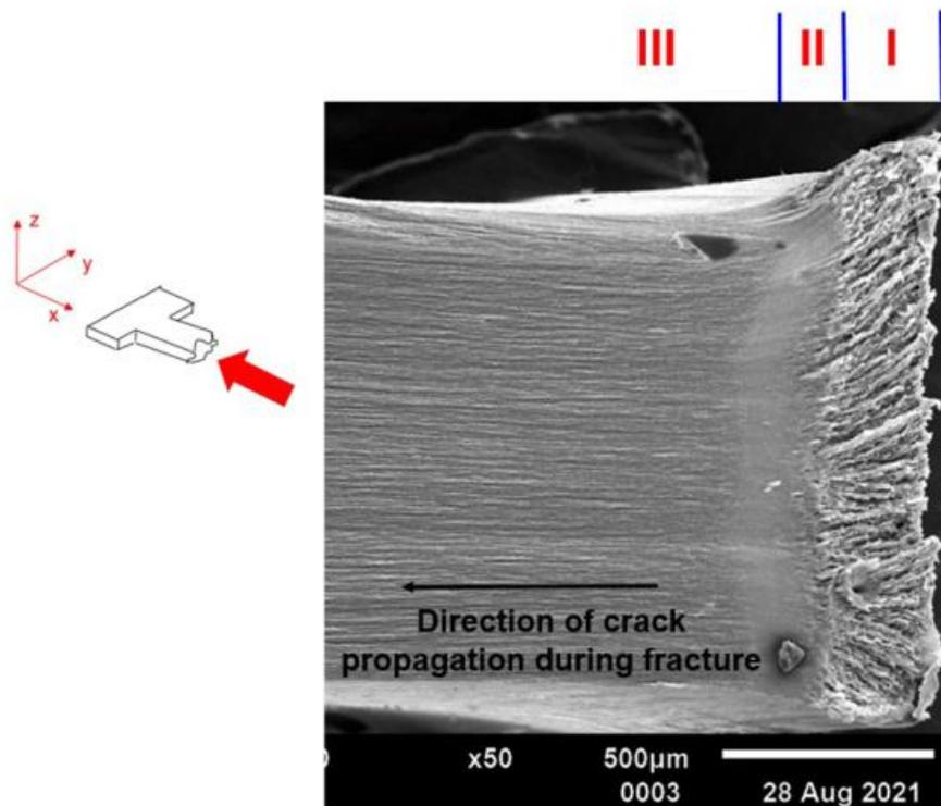
Figure 2: Overall view of fracture surface of cross-rolled HPDE fractured in tension. Three distinct zones associated with different propagation speeds were observed.
