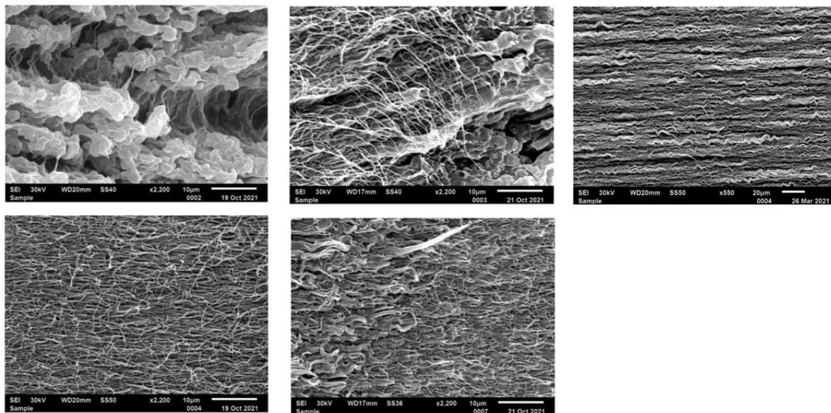
Figure 3: Magnified images of fracture surface, including a) the damage zone (top left), b) the transition between the damage zone and initial fracture zone (top center), c) the bulk slow crack propagation zone (bottom left), d) the transition between the slow and fast crack propagation zone (bottom center), and e) the zone of rapid crack propagation (top right).
