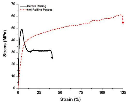
Figure 1: Engineering stress-strain curves of un-rolled and rolled HDPE when pulled in tension to failure at -40 C and a strain rate of 100%/min.
