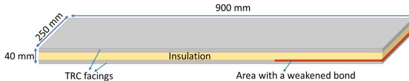
Fig 1. Illustration TRC sandwich beam with destroyed bond.
