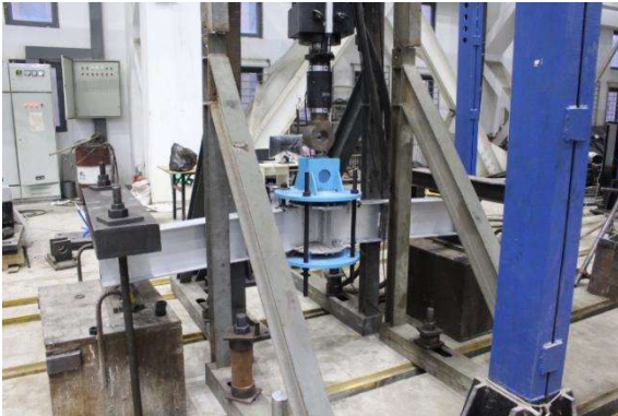
Fig.1 – Experiment of the aluminum alloy joint.
