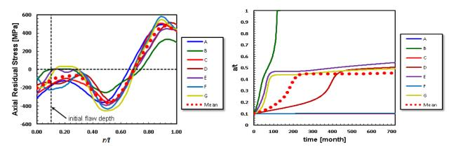
Fig.1 – Example of WRS predictions and associated crack growth predictions: Predictions D, E, and G adequately approximate the mean prediction.
