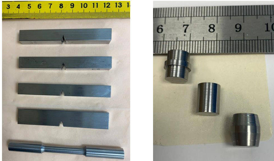
Figure 2 - Left) H13 specimens with V-notches of 30°; 60° and 90° . Right) H13 specimens for experiments required by a triaxiality fracture theorem.
